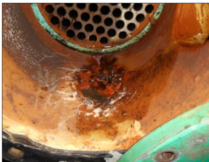
Figure 1. Inside the head of a heat exchanger showing failure of epoxy internal protective coating
