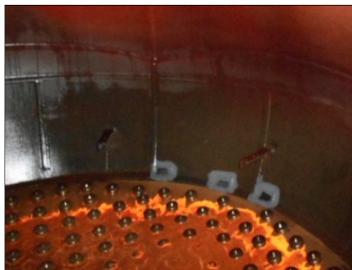
Figure 3. Rubber lined polishing vessel showing localised repairs where the lining was blistered
