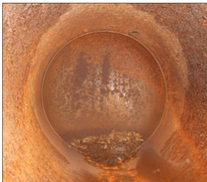
Figure 7. Air receiver showing extensive internal corrosion due to unprotected surfaces
