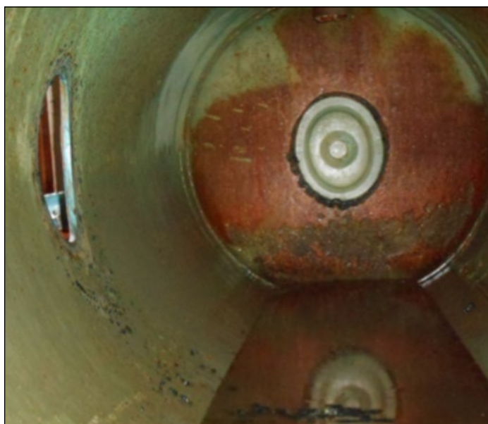
Process vessel showing corrosion at internal surfaces where protective coating has failed
