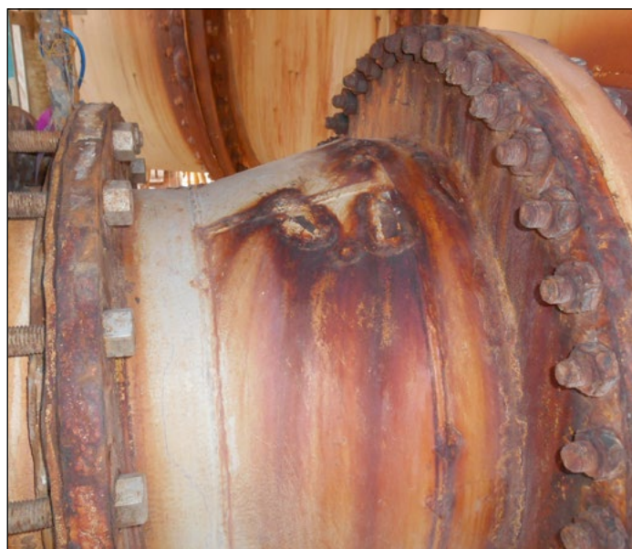
Prominent corrosion due to protective coating failure by chemical attack and harsh environment
